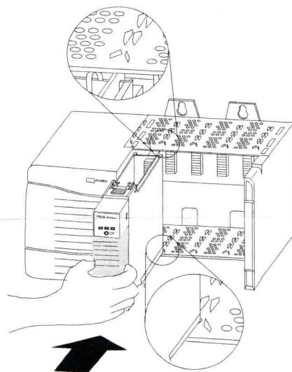
2. Slide the module into the chassis. Make sure the top and bottom locking tabs snap into place.
