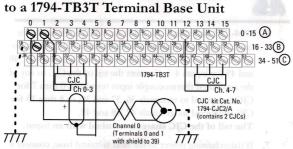
When using grounded thermocouples, and the error is off the same amount on each thermocouple, connect terminal 16 to ground, and connect the thermocouple ground to the same ground,
