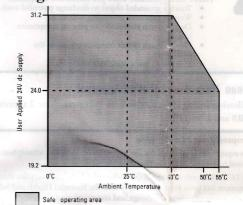
The area within the curve represents the safe operating range for the module under various conditions of user supplied 24V dc supply voltages and ambient
